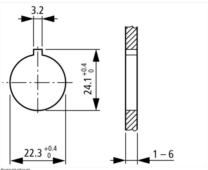
Mounting hole with lug slot
