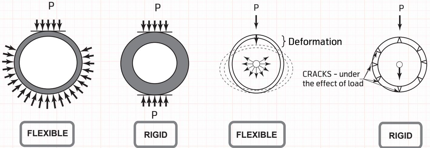
Soil reactions - load distribution for flexible and rigid structures: pipe-soil interaction.
