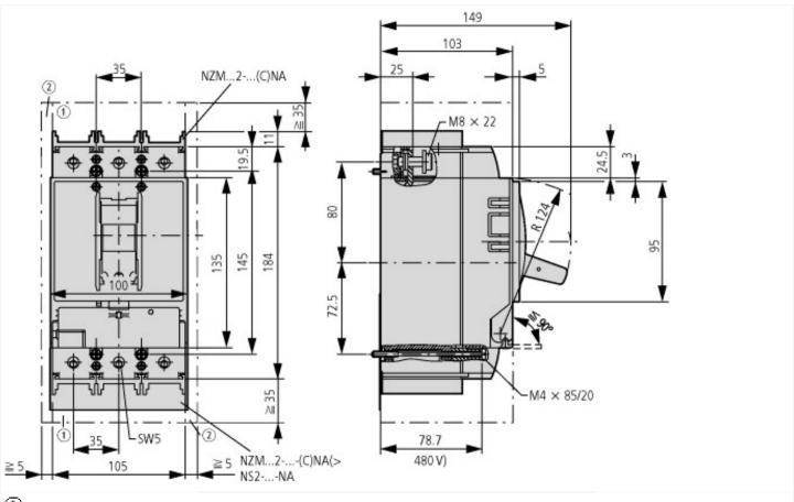
$\underbrace{ \textbf{1}}_{\text{Blow out area, minimum clearance to other parts}}$
